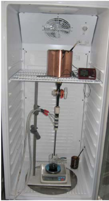
Fig.1 Device for testing Changqing crude oil and crude oil from Venezuela.
