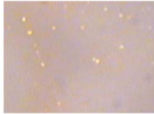
Fig.4 Many micrometer-scale broken DRA polymers inside the crude oil sample.
